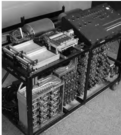
Reconstruction of Atanasoff's computer.
